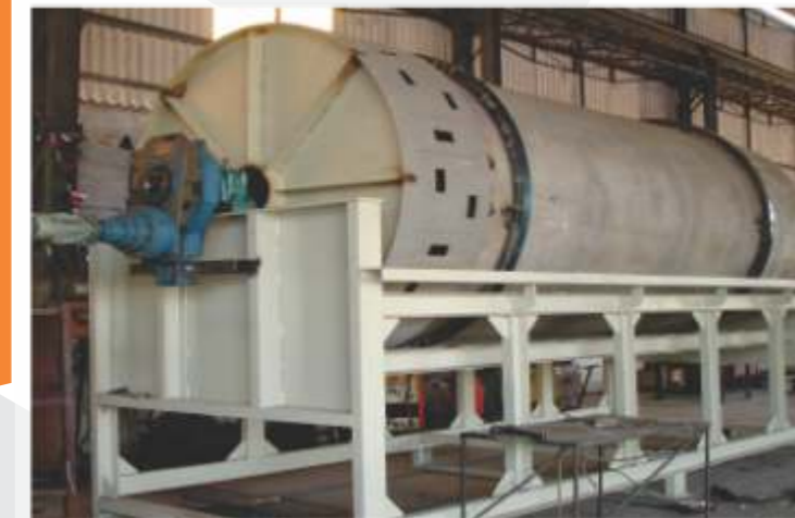
Rotary Drum Dryer
